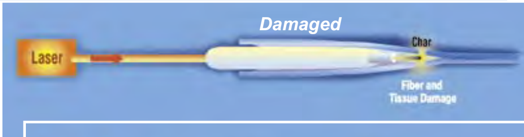
No LPS Feedback Fiber tip starts to char, absorbing laser light and producing unwanted damaging heat.
